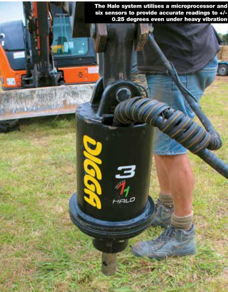
The Halo system utilises a microprocessor and six sensors to provide accurate readings to +/- 0.25 degrees even under heavy vibration
